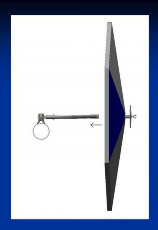
6. INSERT ROOF SECTION INTO ALUMINUM ANGLE BOOM, SECURE WITH PIN
